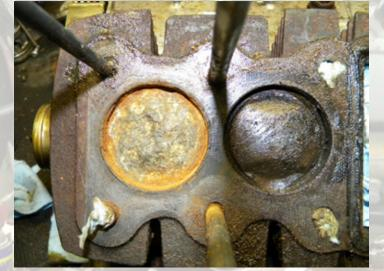
Looks like you could put a lunar lander down on that one! This operation ultimately took a cold chisel and a LOT of penetrant, heat, muscle and time to finally get to budge, and in the end I wound up replacing the head, although I DID manage to get the pistons out.
